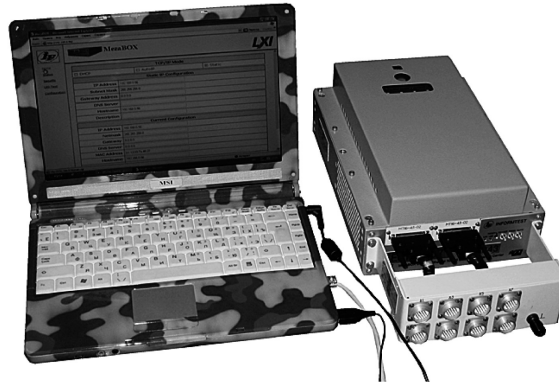
Fig. 2. Dynamic parameter logging device Test-BMP1.
