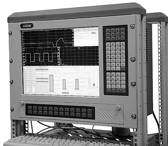
Fig. 5. Bench-test automation system based on ATest package.
